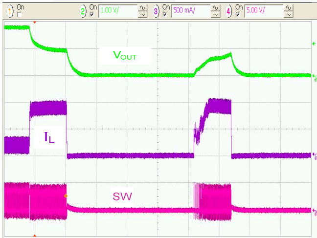
Figure 35. Over-Current Fault Response, R_{LOAD} = 1\Omega , 20\mu s/div.
