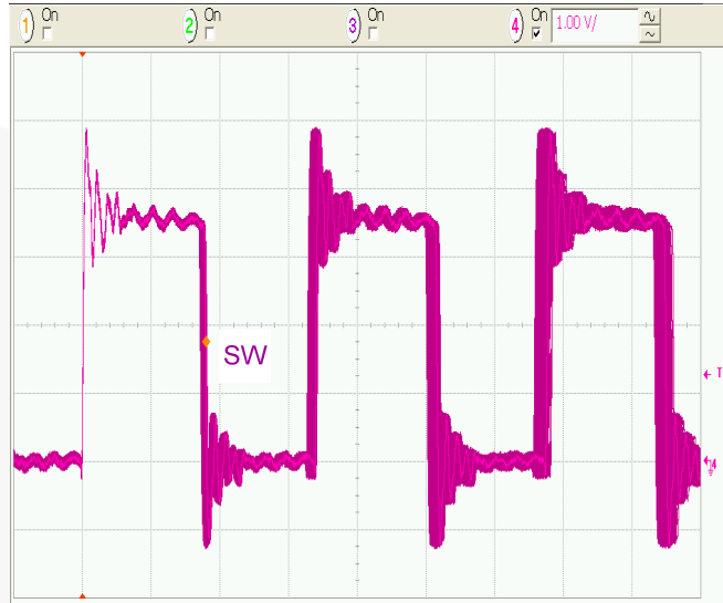
Figure 39. SW-Node Jitter (Infinite Persistence), I_{LOAD} = 200mA , 50ns/div.
