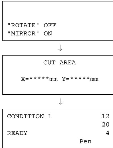
The plotter is now ready to receive data for cutting or plotting. If the interface or command settings have not been made, make these settings before sending the data. If the settings have been made, pen adjustment is performed. When the pen adjustments have been made, the plotter is ready to start cutting. Send the cutting or plotting data from the application software.
