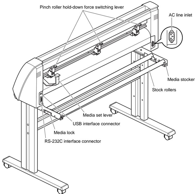
Media set lever: .....Used to raise or lower the pinch rollers during the loading or unloading of media.
