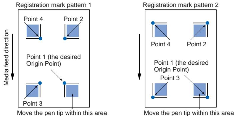
When Point 1 has been scanned, move the pen tip to MARK 2 (within the Point 2 area) then to MARK 3 (within the Point 3 area), and finally to MARK 4 (within the Point 4 area), and perform the same operation as for Point 1.
