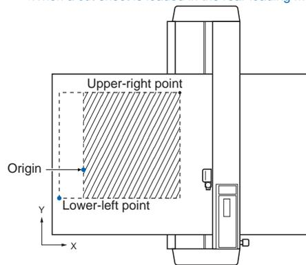
When ROTATE has been selected to rotate the coordinate axes by 90° as shown in the example below, the shaded area represents the effective cutting/plotting area defined by the LL and UR points.
