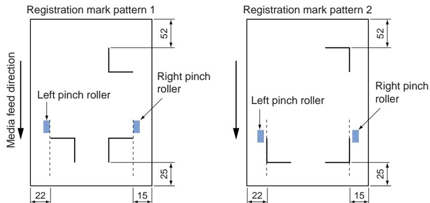
With roll media, the registration marks must be at least 110 mm from the back edge of the media.
