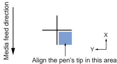
The plotter scans the pre-printed cross mark, and then plots a second cross mark (see the figure below).
