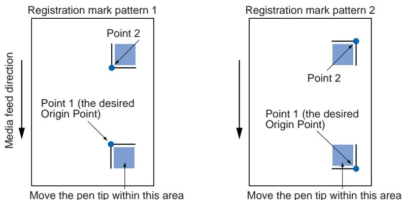
When Point 1 has been scanned, move the pen tip to MARK 2 (within the Point 2 area) and then perform the same operation as for Point 1.
