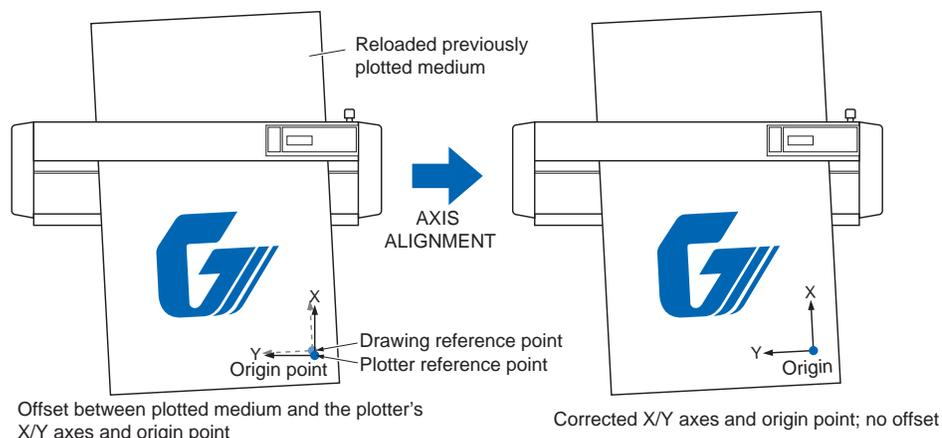
Cutting is performed after alignment has been performed for the origin point and the X and Y axes of the previously plotted medium, or for the registration mark reference point, to eliminate any offset. When performing axis alignment, use media with a grid or printed registration marks to enable the X and Y axes and the origin point to be determined.
