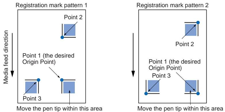
When Point 1 has been scanned, move the pen tip to MARK 2 (within the Point 2 area) and then to MARK 3 (within the Point 3 area), and perform the same operation as for Point 1.
