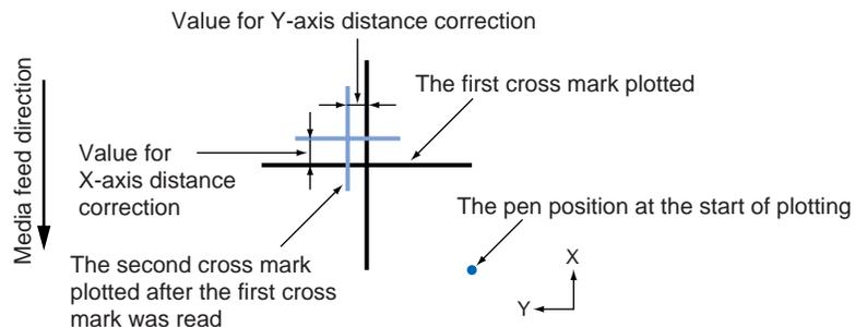
After the cross mark is read, use the pen for which Pen Condition 1 was specified to draw a second cross mark.
