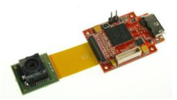
A DMA channel on the FPGA is used to read the data and send it to the USB 3.0 channel.
