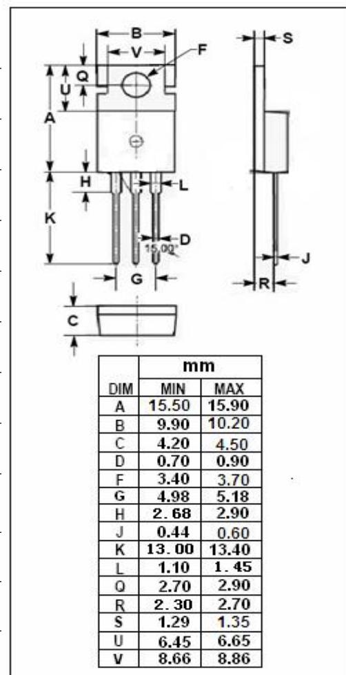
**isc N-Channel MOSFET Transistor****FCP125N65S****ELECTRICAL CHARACTERISTICS****T<sub>c</sub>=25°C unless otherwise specified**
