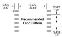
Dimensions are in  $\frac{\text{inches}}{\text{mm}}$
