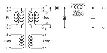
The primary windings and the secondary windings are to be connected in parallel on the PC board.
