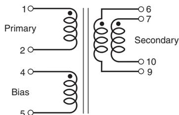
Secondary windings to be connected in parallel on PCB board.
