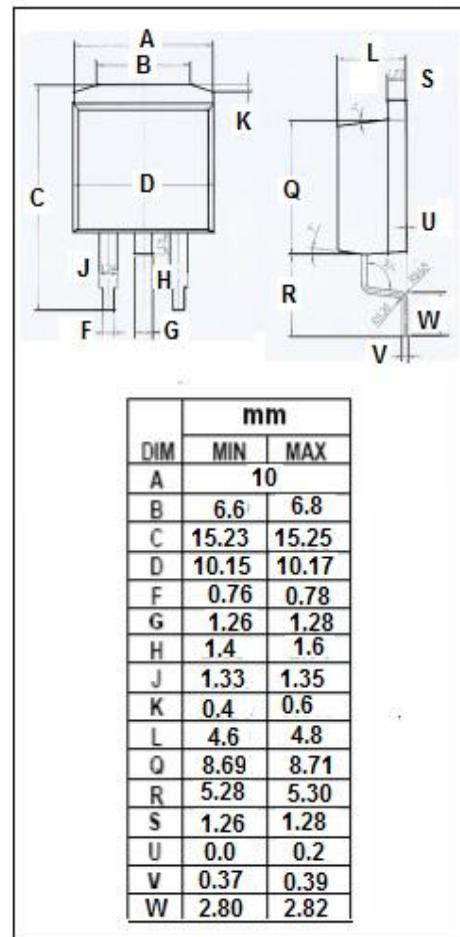
**Isc N-Channel MOSFET Transistor****FDB075N15A****ELECTRICAL CHARACTERISTICS** $T_c=25^\circ\text{C}$  unless otherwise specified
