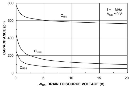
Figure 8. Capacitance Characteristics.
