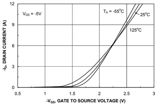
Figure 5. Transfer Characteristics.
