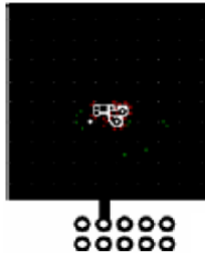
a) 86 °C/W when mounted on a 1 in 2 pad of 2 oz copper.
