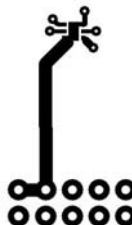
d. 151^\circ\text{C}/\text{W} when mounted on a minimum pad of 2 oz copper
