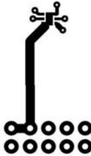
d. 151\text{ }^\circ\text{C/W} when mounted on a minimum pad of 2 oz copper
