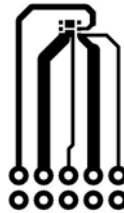
b. 173\text{ }^\circ\text{C/W} when mounted on a minimum pad of 2 oz copper
