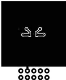
a. 57°C/W when mounted on a 1 in<sup>2</sup> pad of 2 oz copper
