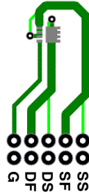
b) 125°C/W when mounted on a minimum pad
