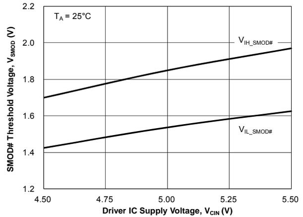
Figure 19. SMOD# Threshold vs. Driver Supply Voltage
