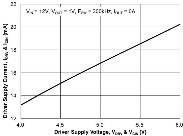
Figure 14. Driver Supply Current vs. Driver Supply Voltage
