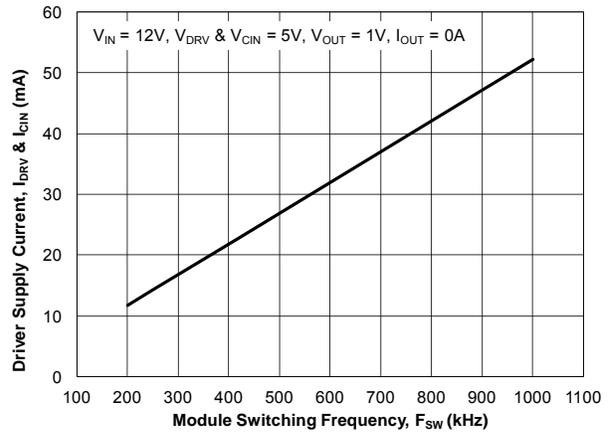
Figure 13. Driver Supply Current vs. Switching Frequency
