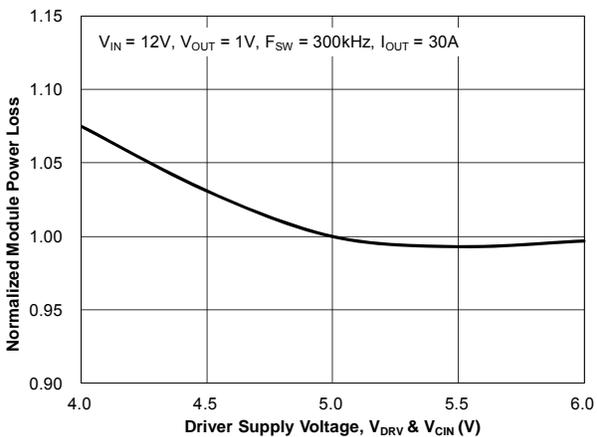
Figure 10. Power Loss vs. Driver Supply Voltage
