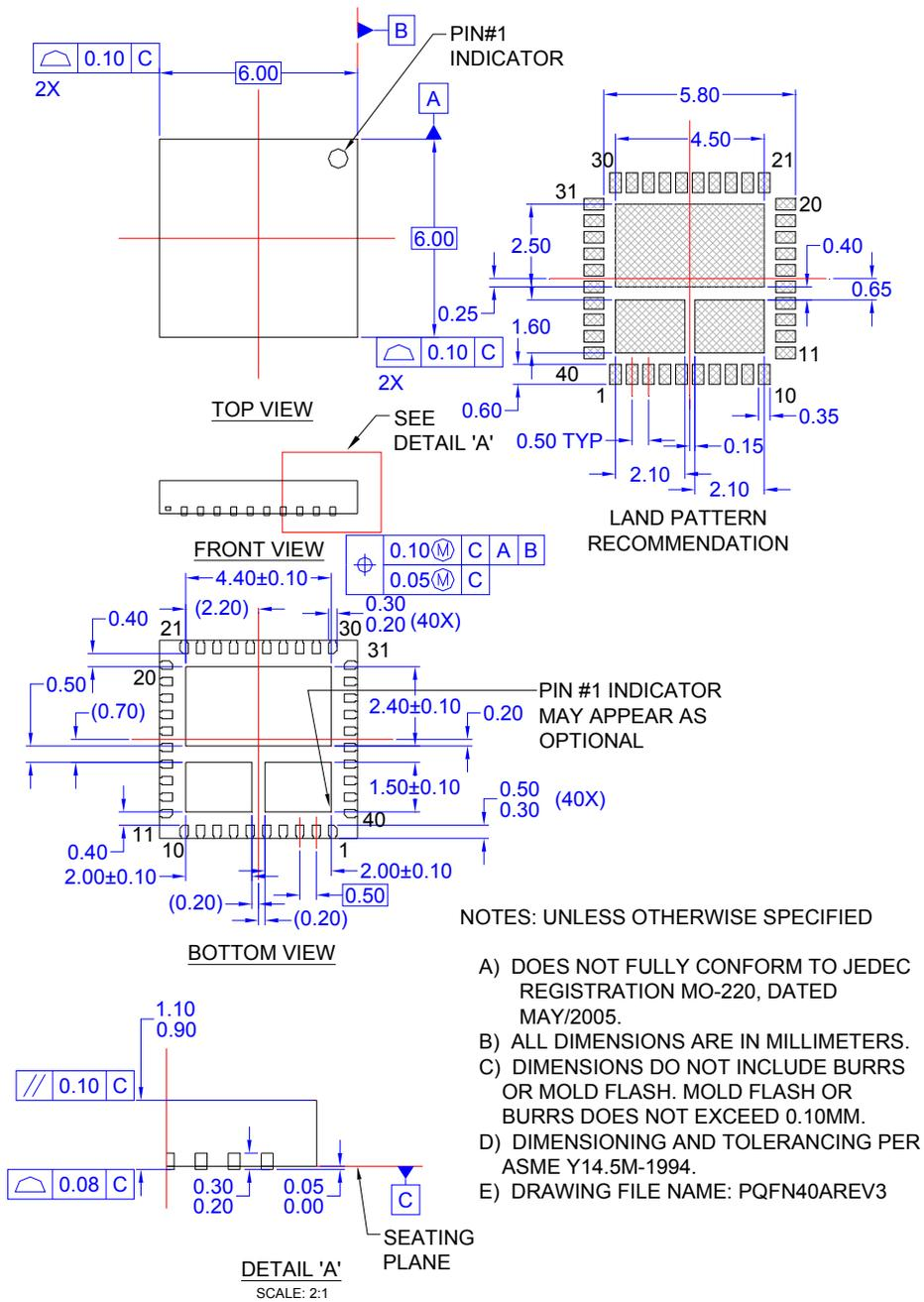
**Figure 33. 40-Lead, Clipbond PQFN DrMOS, 6.0x6.0 mm Package**
