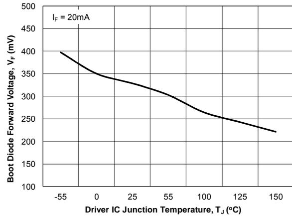
**Figure 25. Boot Diode Forward Voltage vs. Temperature**
