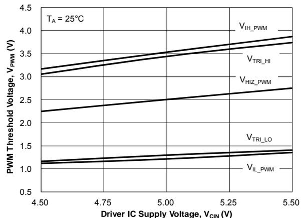
Figure 17. PWM Threshold vs. Driver Supply Voltage
