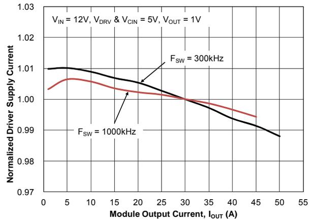
Figure 15. Driver Supply Current vs. Output Current
