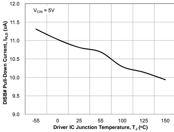
**Figure 24. DISB# Pull-Down Current vs. Temperature**
