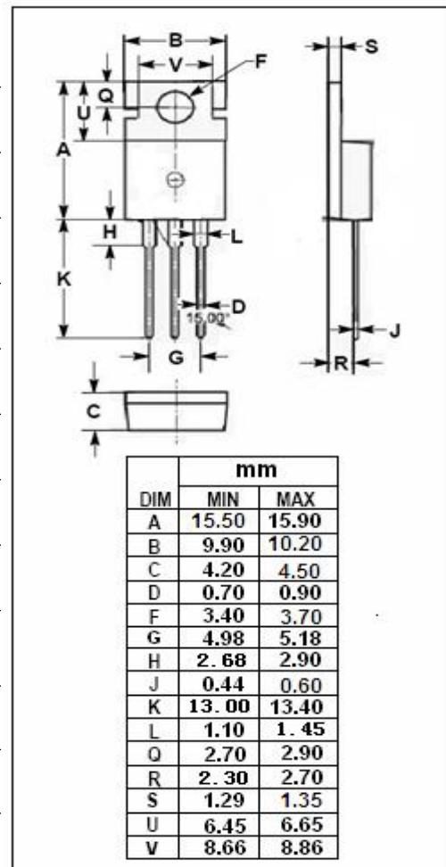
**isc N-Channel MOSFET Transistor****FDP085N10A****ELECTRICAL CHARACTERISTICS****T<sub>c</sub>=25°C unless otherwise specified**
