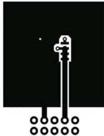
a) 50\text{ }^\circ\text{C}/\text{W} when mounted on a 1\text{ in}^2 pad of 2 oz copper.
