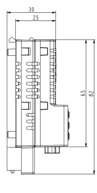
**Mounting:** Into the option slot on the drive.
