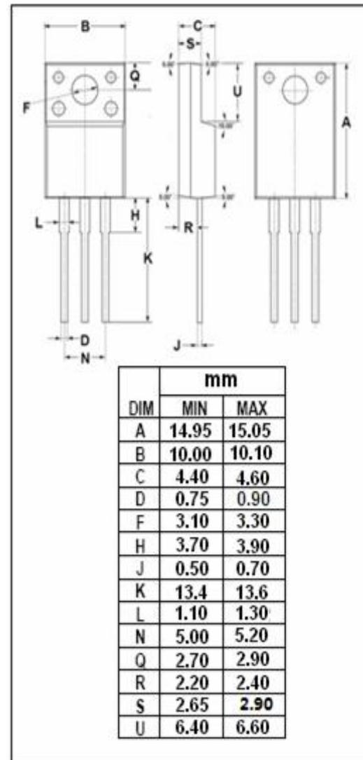
**isc N-Channel MOSFET Transistor****FKV575****ELECTRICAL CHARACTERISTICS** $T_C=25^{\circ}\text{C}$  unless otherwise specified
