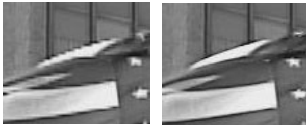
Fig. A2. Conventional vertical interpolation on diagonal edges (L) versus diagonal interpolation (R)
