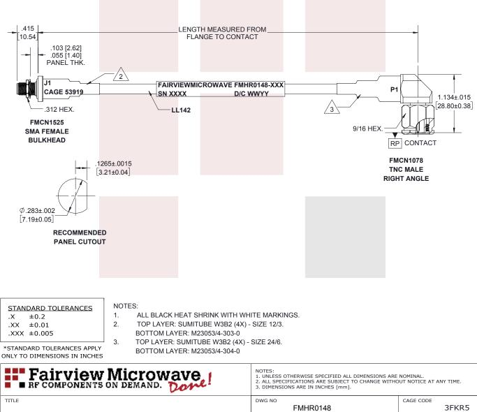
Temperature Conditioned Low Loss SMA Female Bulkhead to RA TNC Male Cable LL142 Coax
