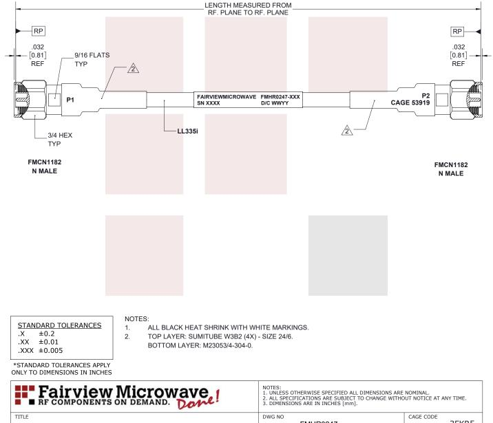
Temperature Conditioned Low Loss N Male to N Male Cable LL335i Coax
