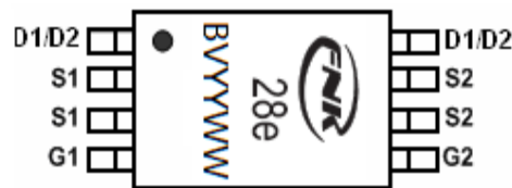
Marking and pin Assignment
