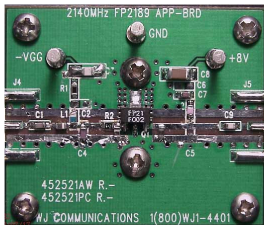
14 mil GETEK™ ML200DSS ( \epsilon_r = 4.2 ) The main microstrip line has a line impedance of 50 \Omega .
