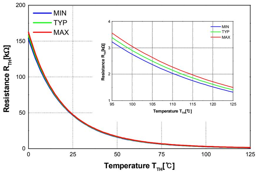
Fig. 9. R-T Curve of the Built-in Thermistor
