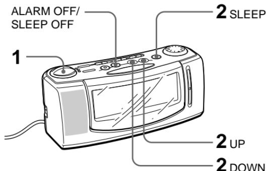
You can use the sleep timer to turn the radio off automatically after up to 59 minutes.
