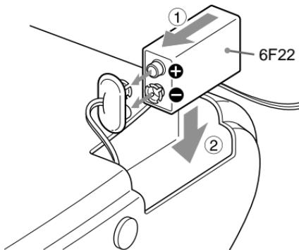
If the AC power supply is interrupted, the clock display goes off and the alarm setting is canceled. To back up the clock and alarm, insert a 6F22 battery in the battery compartment on the rear of the unit. → **A**
