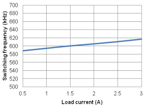
Figure 8. Switch Frequency vs. Load Current
