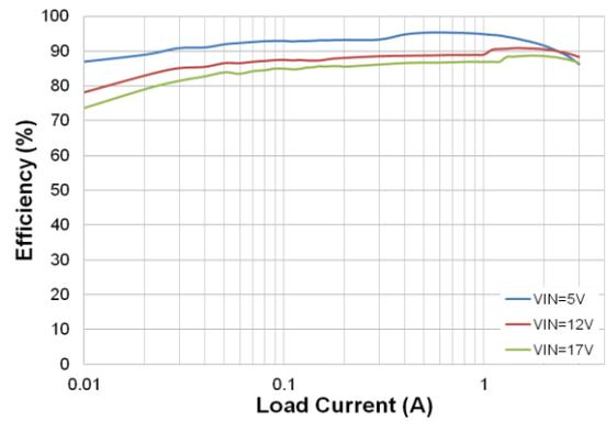
Figure 5. Efficiency vs. Load Current
