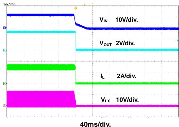
Figure 15. Shutdown Through Power Supply Waveform
