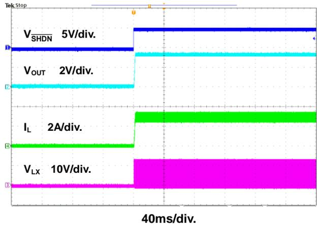
Figure 17. Startup Through  $\overline{SHDN}$  Waveform
