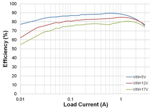
Figure 4. Efficiency vs. Load Current
