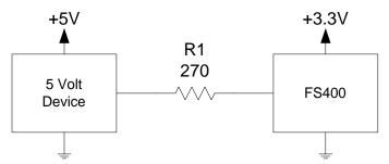
Figure 23. 5 to 3.3 Volt Translation using a Resistor
