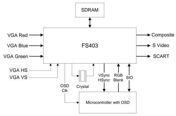
Figure 1: External Scan Converter Block Diagram
