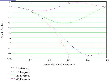
Figure 10: FLK = 16, SHP = 16; Response at Horizontal, 14, 27, 45 Degrees
