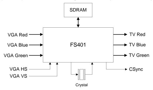
Figure 2: Embedded Television Design Block Diagram
