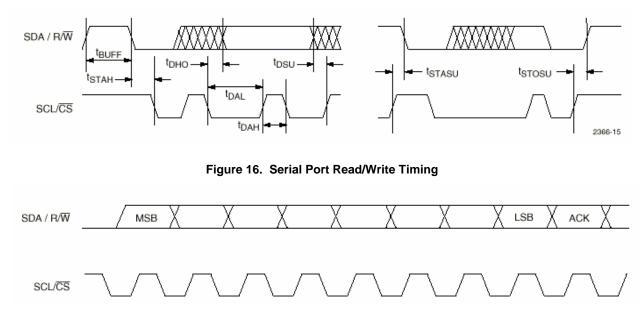
Figure 17. Serial Interface – Typical Byte Transfer
