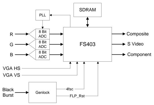
Figure 4: Professional & Pro-Consumer Video Design Block Diagram
