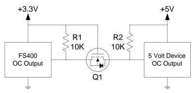
Figure 27. SIO (Open Collector) Translation using a MOSFET Q1 = BSS138
