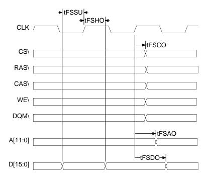
Figure 11. Timing Parameter Definition, SDRAM Interface
