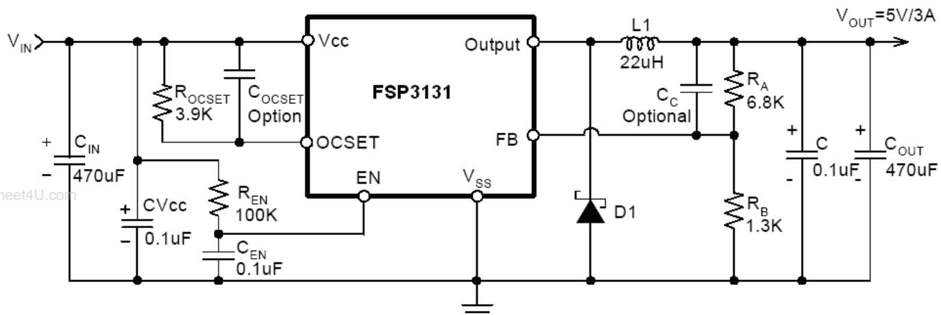
Note:  $V_{OUT} = V_{FB} * (1 + R_A/R_B)$
