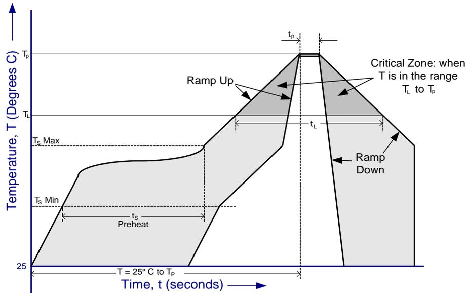
**Figure 11.5 FT201X Solder Reflow Profile**
