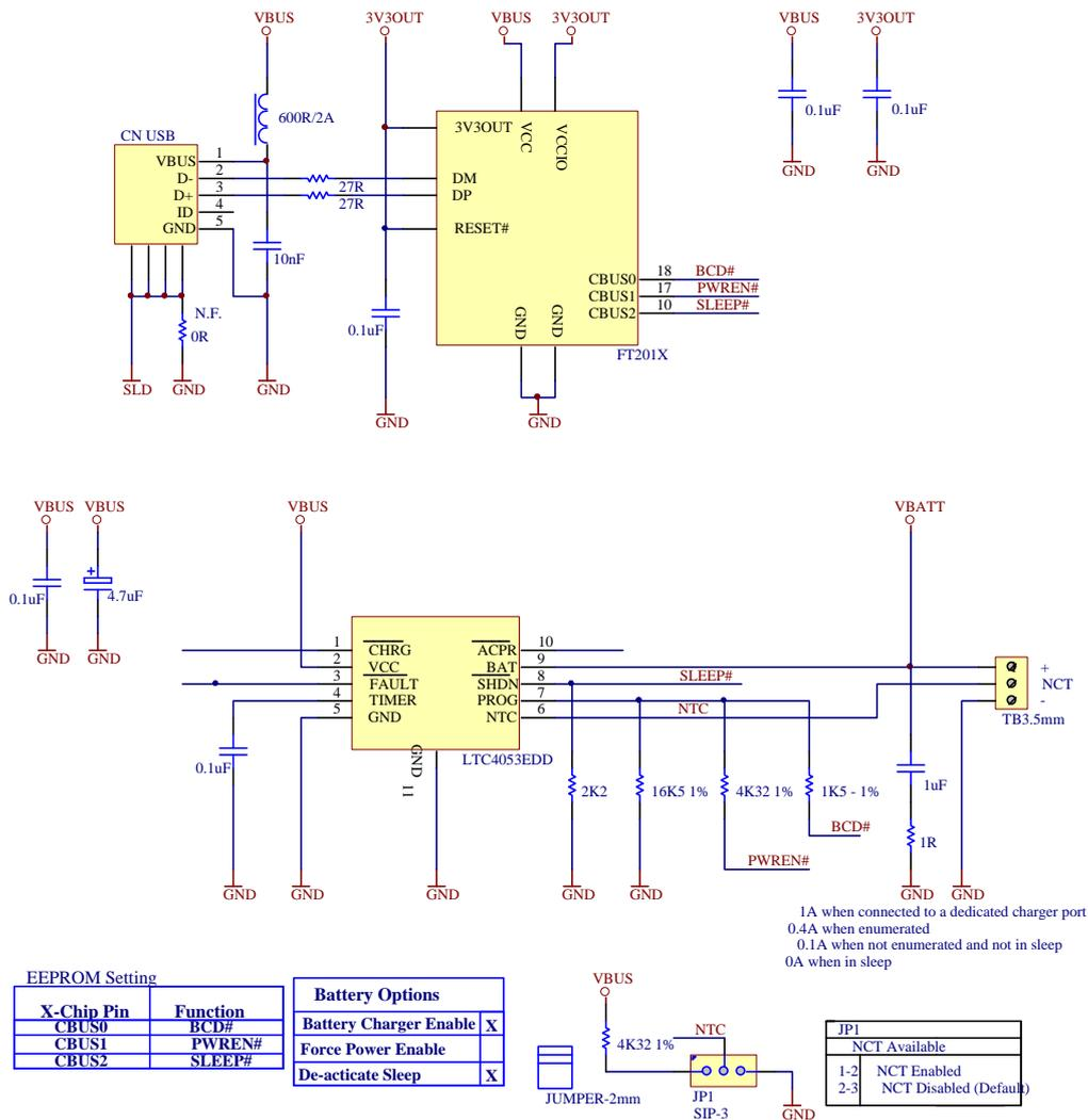
**Figure 8.4 USB Battery Charging Detection (3 - pin)**
