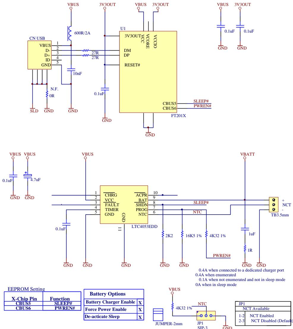
**Figure 8.3 USB Battery Charging Detection (2- pin)**
