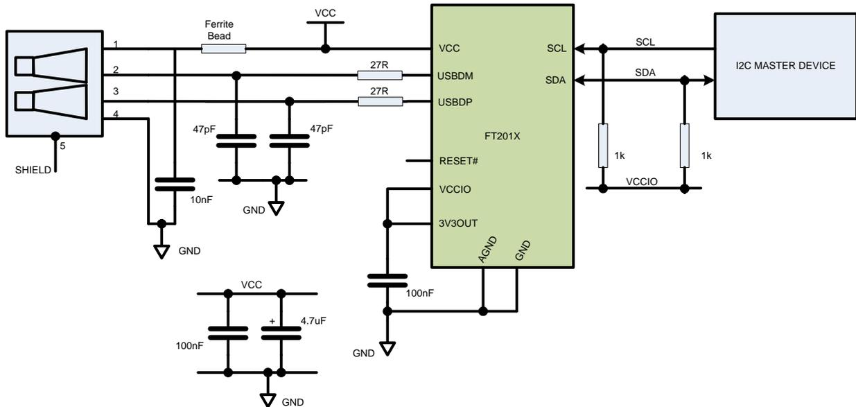
**Figure 8.1 Application Example showing USB to I<sup>2</sup>C Converter**
