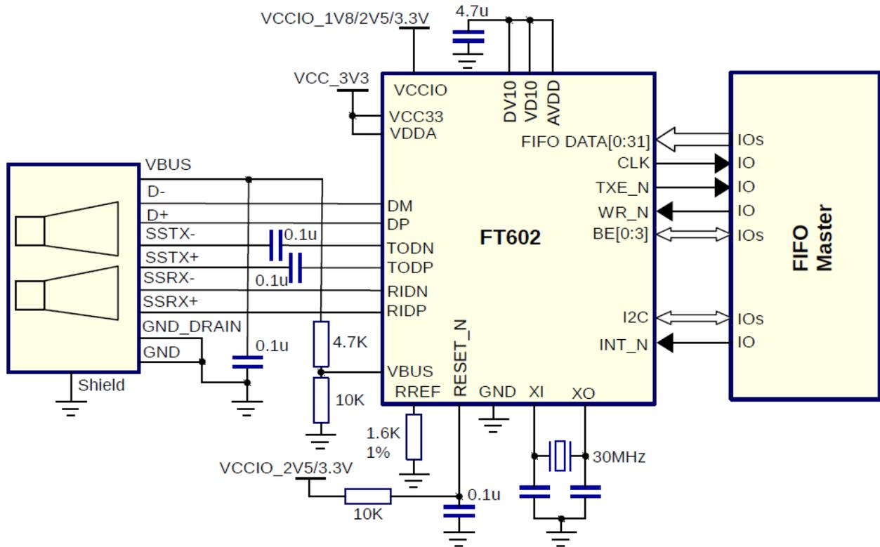
**Figure 7.2 FT602 Connect to FIFO Master Interface (245 Synchronous FIFO Mode)**
