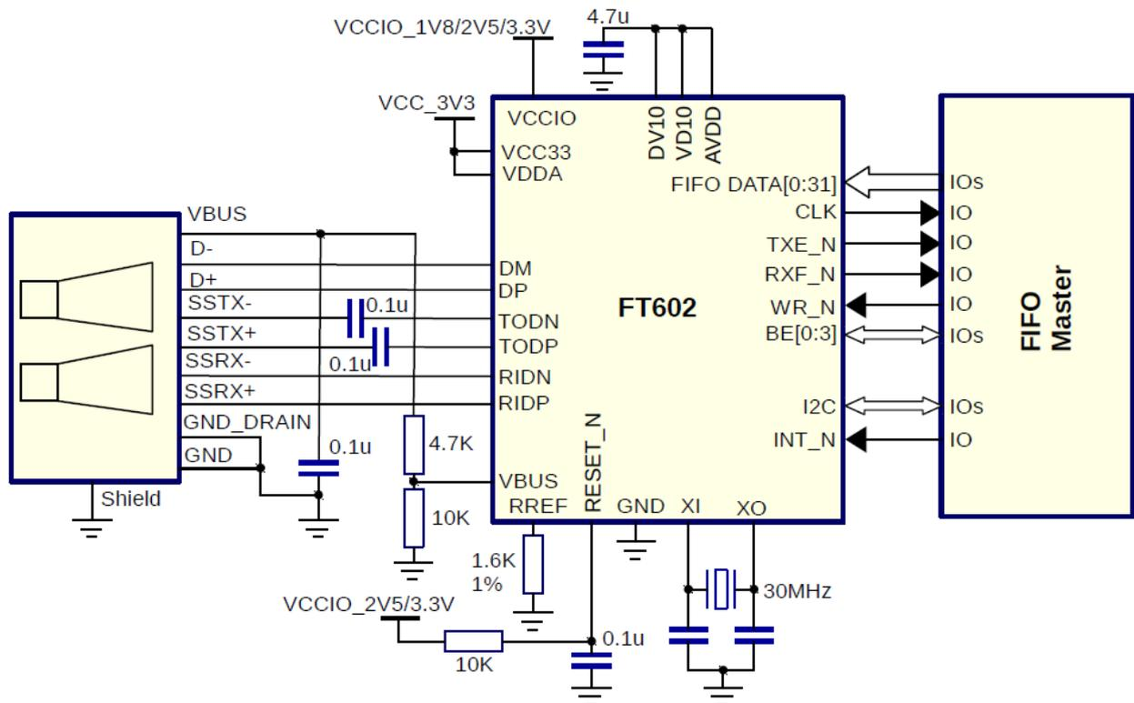
**Figure 7.1 FT602 Connect to FIFO Master Interface (Multi-Channel FIFO Mode)**
