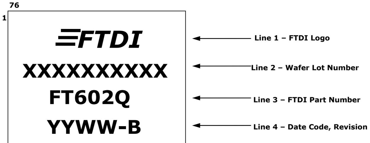
**Figure 8.2 QFN-76 Package Markings**
