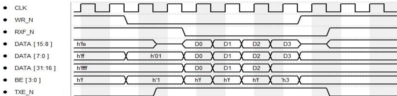
**Figure 4.1 Multi-Channel FIFO mode master write transaction 1**
