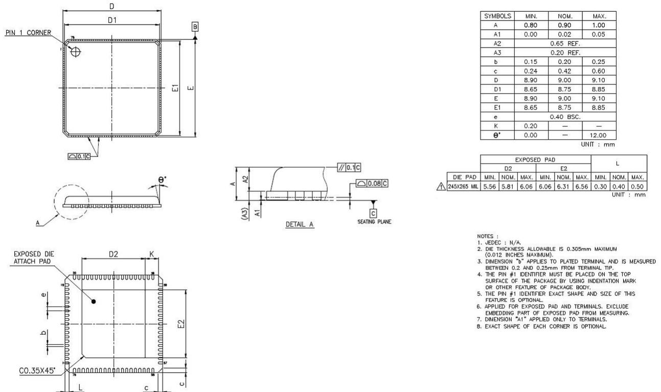
**Figure 8.1 QFN-76 Package Dimensions**
