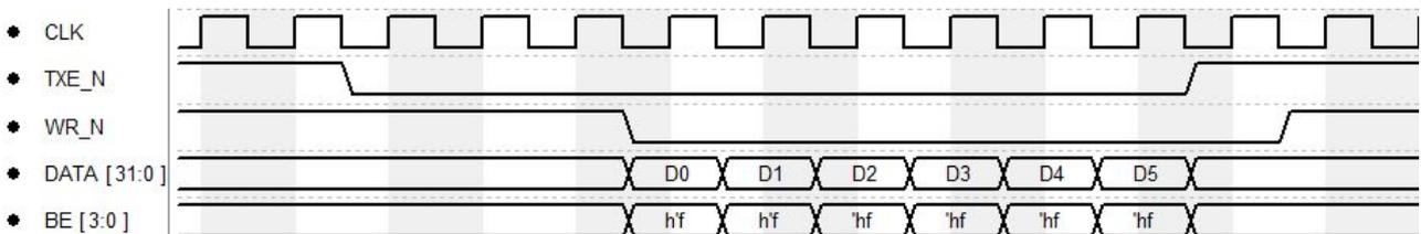
**Figure 4.3 245 Synchronous FIFO mode bus master write cycle**
