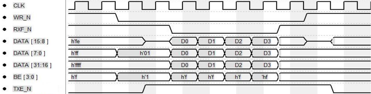
**Figure 4.2 Multi-Channel FIFO mode master write transaction 2**
