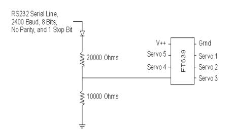
Note: For a serial line that has voltage from 0 to V++ requires no diode resistor network. The line can be connected directly to the serial-in pin on the FT639.
