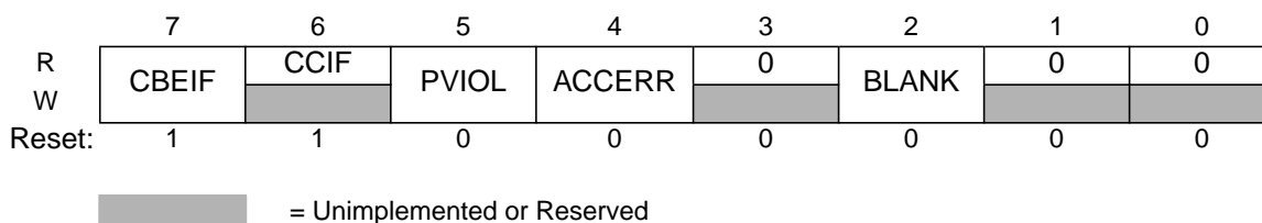
Figure 3-7 Flash Status Register (FSTAT)
