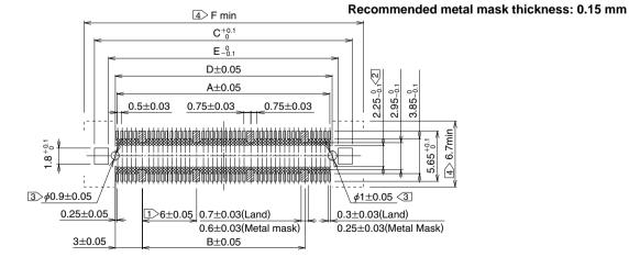
Note  $\square$  Cross-hatched portions, totaling n places, indicate the ground circuits.
