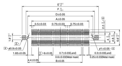
Note  $\square$  Cross-hatched portions, totaling n places, indicate the ground circuits.
