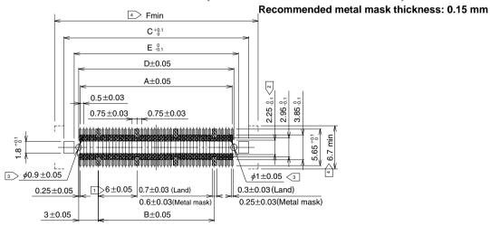
Note Cross-hatched portions, totaling n places, indicate the ground circuits.
