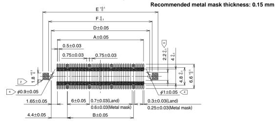
Note  $\square$  Cross-hatched portions, totaling n places, indicate the ground circuits.
