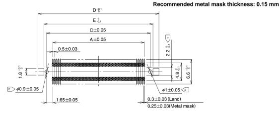
Note 1 The cross-hatched area inside the SMT land may come into contact with the connector contacts and thus care should be taken that the pattern does not extend beyond the SMT land width.
