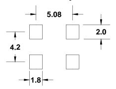
Note: XPRESSO HCMOS XOs are designed to fit or industry standard, 4 pad, layouts.
