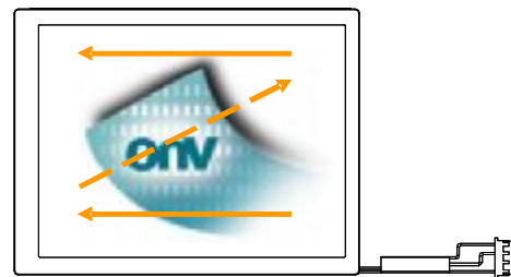
Fig. 2 Reverse scan (Pin19 = High)
