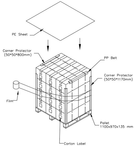
**Figure. 9-2 Packing method**
