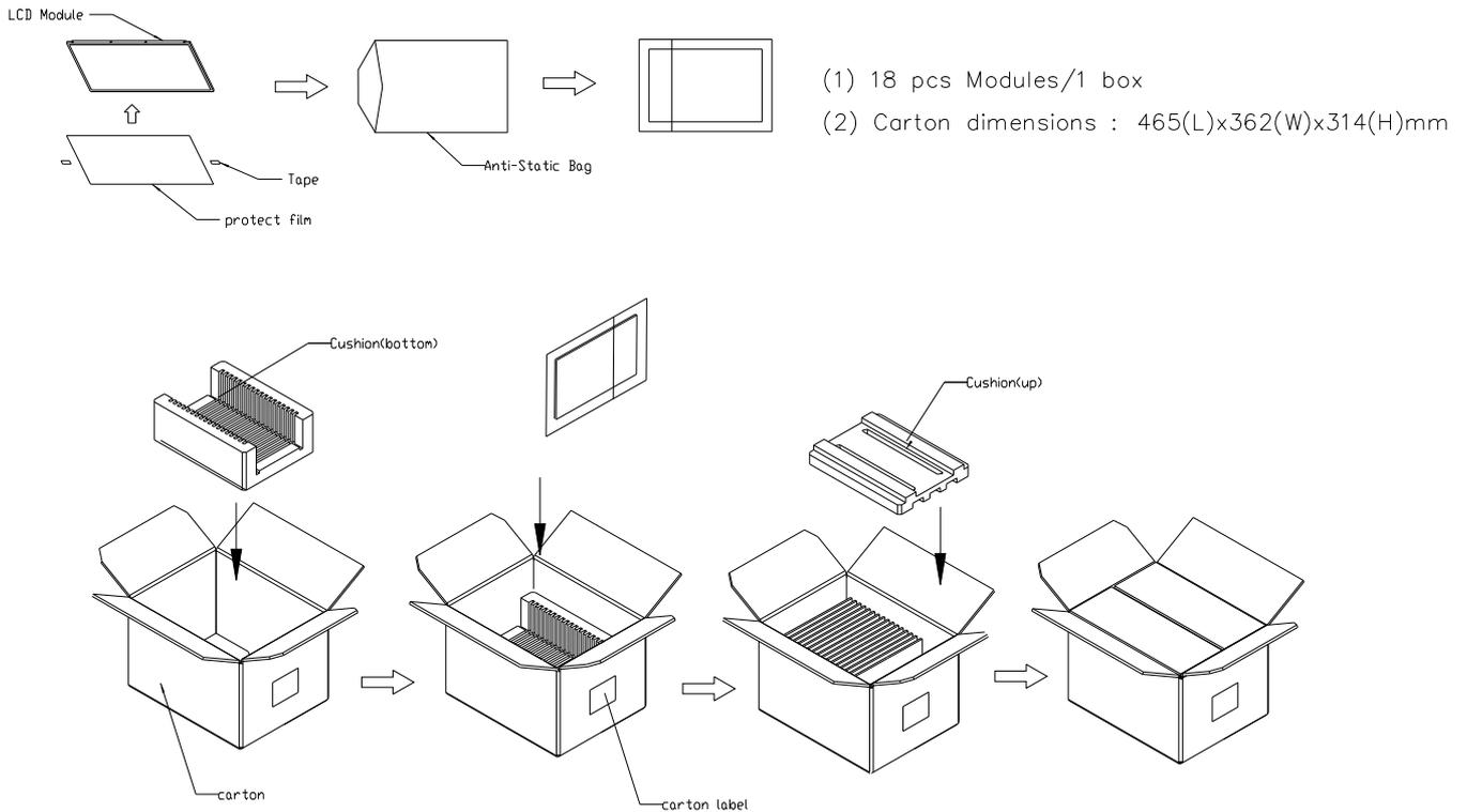
**Figure. 9-1 Packing method**
