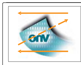
Fig. 2 Reverse scan (Pin19, RSV = High or VDD)
