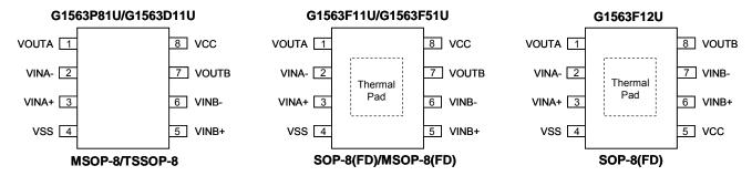
Note: Recommend connecting the Thermal Pad to the VSS for excellent power dissipation.
