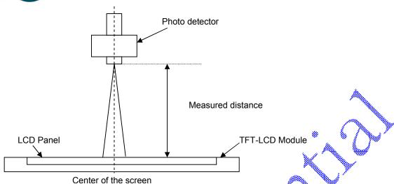
Note 2: Definition of viewing angle measured by ELDIM (EZContrast 88)
