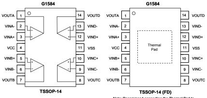
Note: Recommend connecting the Thermal Pad to the Pin#11 VSS for excellent power dissipation.
