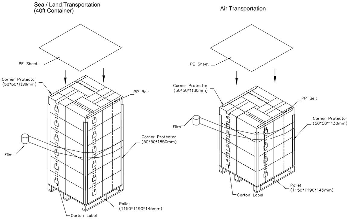
**Figure. 9-2 Packing method**
