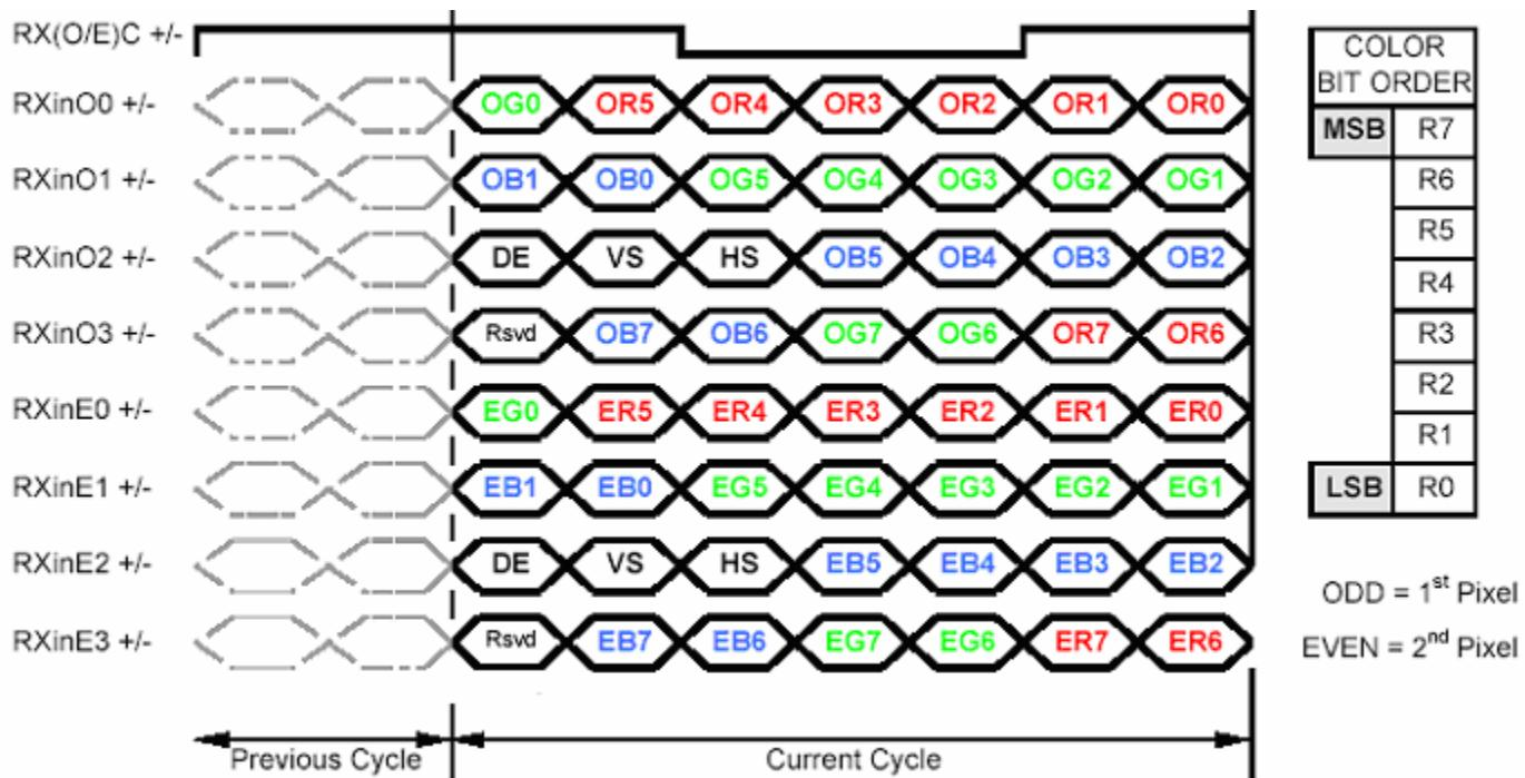
Note1: Normally DE mode only. VS and HS on EVEN channel are not used.
