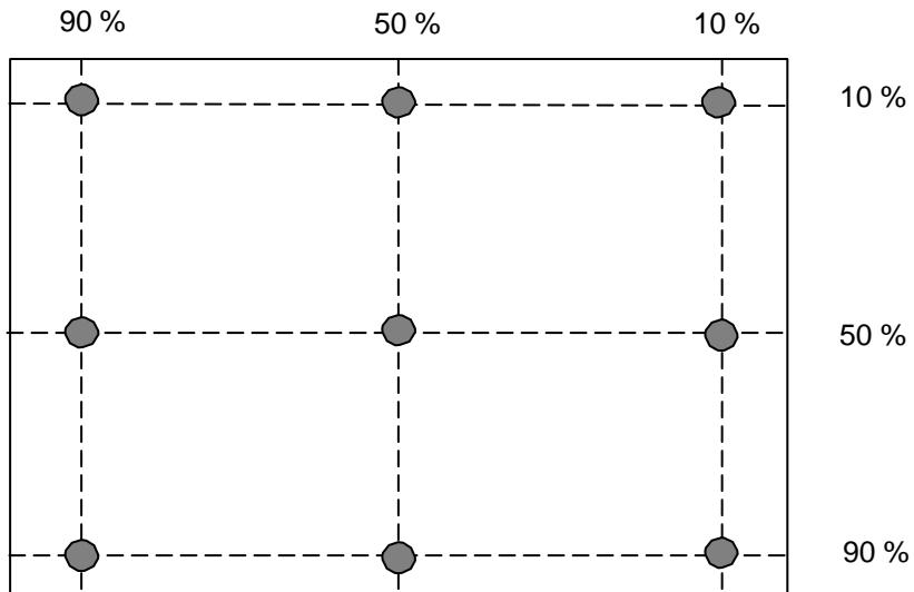
Note 3: The luminance uniformity of 9 points is defined by dividing the maximum luminance values by the minimum test point luminance. And measured by TOPCON SR-3
