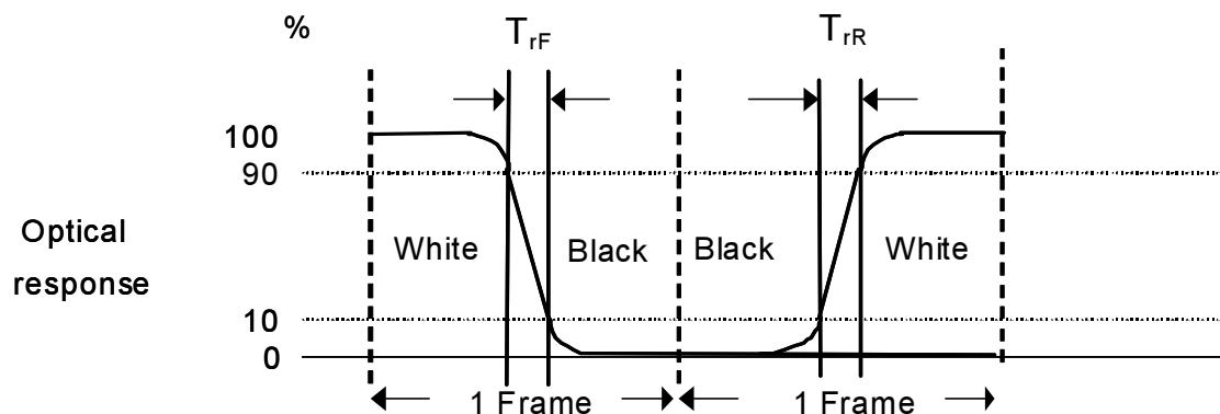
$$T_{rR} + T_{rF} = 5 \text{ msec (typ.)}$$
