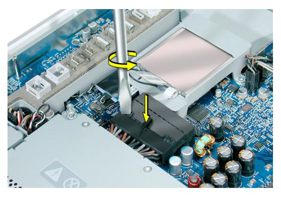
5. Pull on the connector, not on the cables.
