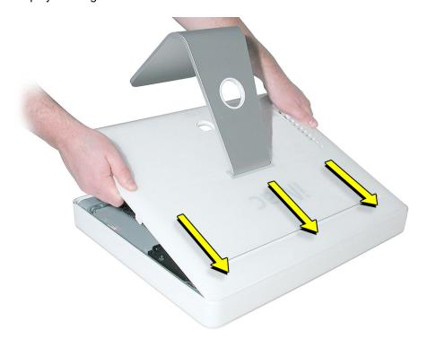
2. Lower and press the cover into place until it fits snugly on the computer.
