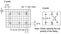
Fully Sealed Model Single Latching Models G6CU-□114P-US
