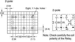
Fully Sealed Double-winding Latching Model G6CK-□114P-US
