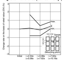
Sample: G6C-2114P-US DC24V Number of Relays: 6 pcs Test conditions: Shock is applied in  $\pm X$ ,  $\pm Y$ , and  $\pm Z$  directions three times each with without energizing the Relays to check the number of malfunctions.
