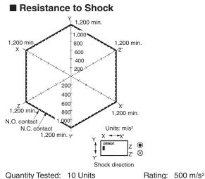
Test Method: Shock was applied 3 times in each direction with and without excitation and the level at which the shock caused malfunction was measured.
