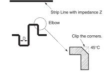
When the lines must curve, an elbow can be used as shown in the diagram. A distance (D) between the lines of approximately twice the line width is sufficient.
