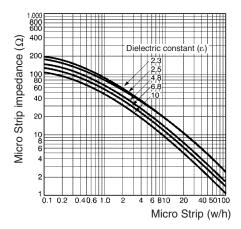
• For example, when creating  $50-\Omega$  lines using a glass epoxy base with a thickness of 1.6 mm, the above graph will yield a w/h ratio of 1.7 for a dielectric constant of 4.8. Since the base thickness is 1.6 mm, the width will be  $h \times 1.7 \approx 2.7$  mm.
