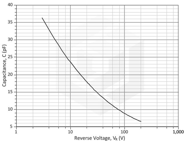
Figure 5: Typical Junction Capacitance versus Reverse Voltage Characteristics
