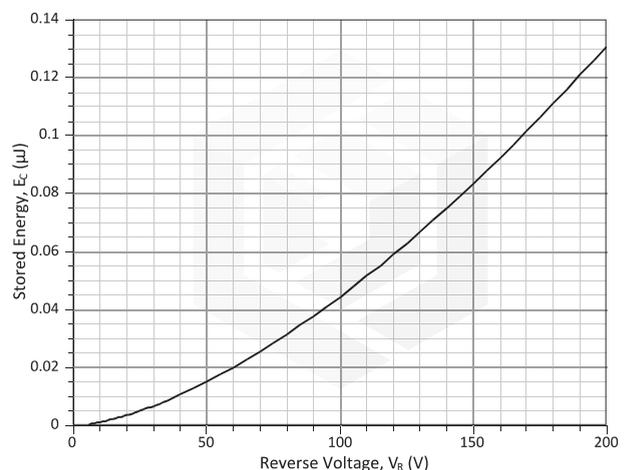
Figure 6: Typical Switching Energy versus Reverse Voltage Characteristics
