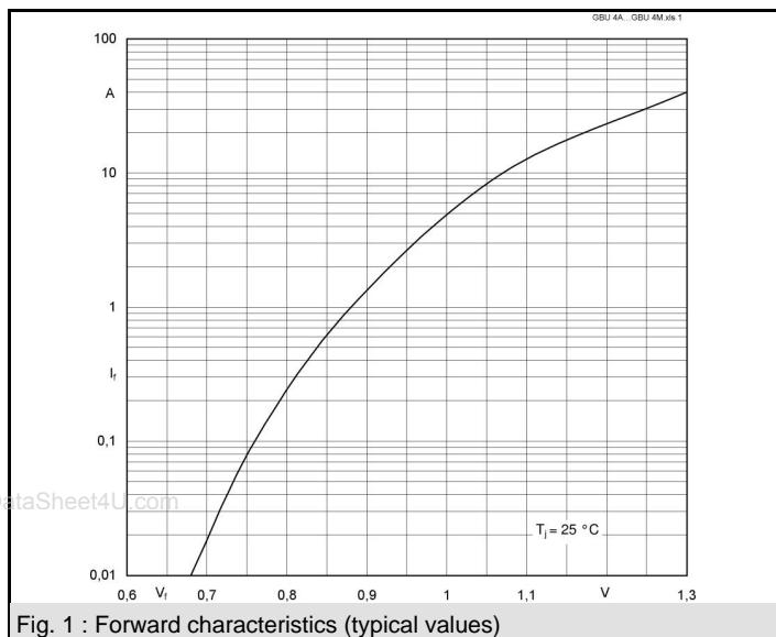
Fig. 1 : Forward characteristics (typical values)
