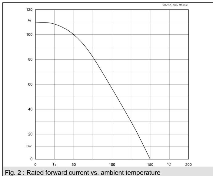
Fig. 2 : Rated forward current vs. ambient temperature
