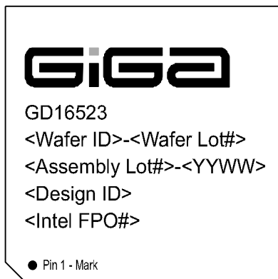
Figure 10. Device Marking. Top View.
