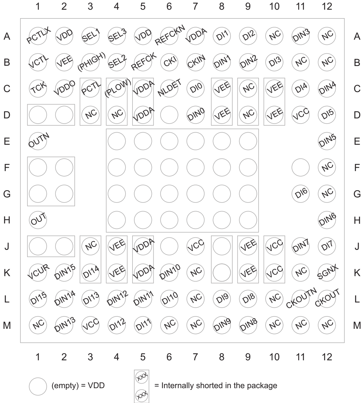
Figure 8. Packages EB and EF Pinout. Top view seen through the package.
